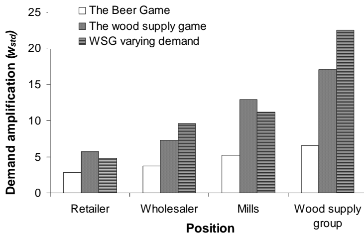
Figure 3. The accumulated demand amplification for the different positions in BG and WSG. Demand amplification is estimated as the standard deviation of the order rates placed by an individual player relative to standard deviation of the initial demand.
